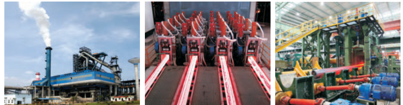
炼铁炼钢生产线 Blast Furnace 弧形连铸圆管坯生产线 Curve Continuous Casters for Round Billet Φ720周期轧管机组 Φ720 Hot Pilger Mill
