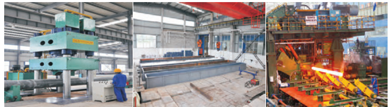
100吨校直机 YF1000 Four-Pillars Hydraulic straightness Machine 酸洗、磷化、皂化生产线 Acid Pickling, phosphating, and saponification line Φ180PQF连轧管机组 Φ180 PQF Mill
