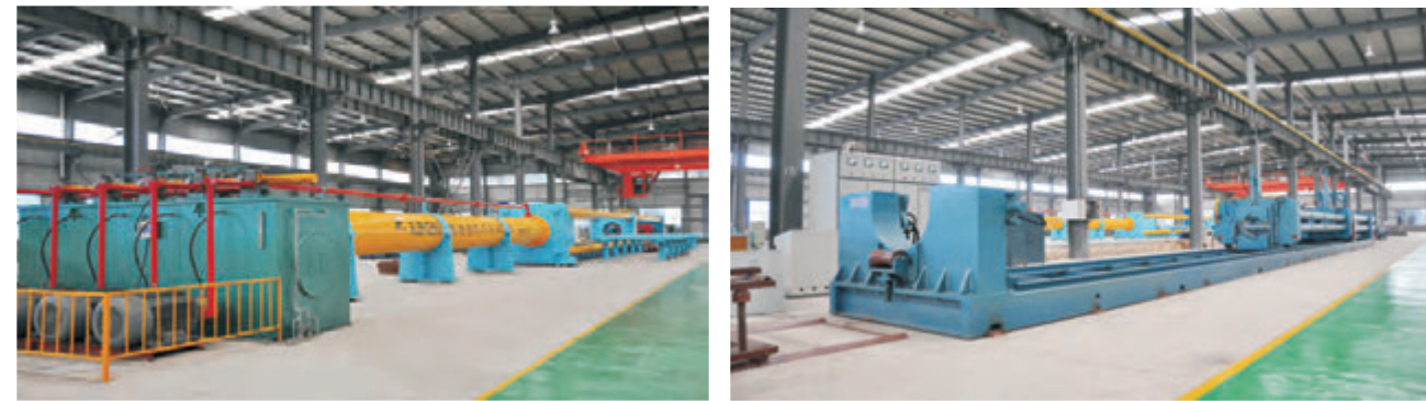
JLB1250T-14500精密冷拔机组 JLB1250T-14500Precision hydraulic cold drawing mill EZG- II B 830X60液压二步推进制管机 EZG- II B Φ830 × 60hot-expanded mill
